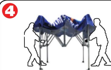
**Step 4:** Fully open the marquee by having a person on each side grasping the lower truss bars and walking backwards.
