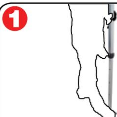
**Step 1:** Pull out the pin and push down on the upper leg to retract. Repeat this step on each leg ensuring all sides are being lowered equally.
