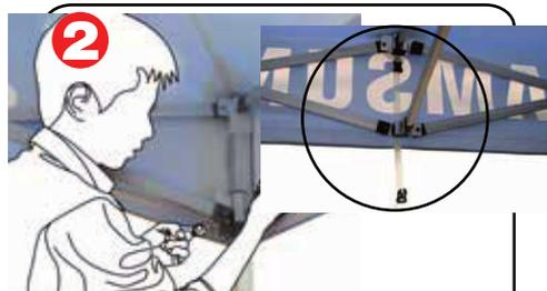
**Step 2:** Unclip all straps and pull out the pin on the upper section of the frame to disengage.
