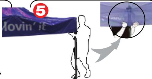
**Step 5:** Push up on truss bars to engage pins.
